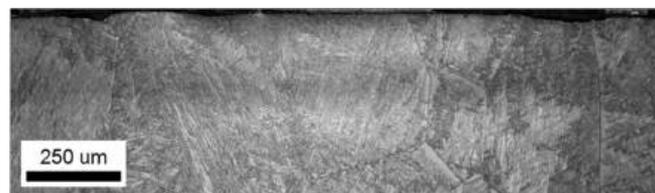
**Figure 4.** Overview EBSD IQ map of the initial material with lamellar microstructure after LSP (the surface is at the top of the micrograph).
