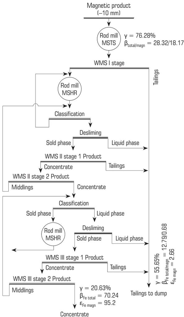
Fig. 4. Recommended processing flowchart for ferruginous quartzite of test deposit
