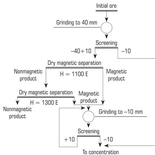
Fig. 1. Ferruginous quartzite pretreatment flowchart with DMS
