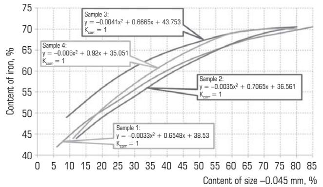
Fig. 5. Effect of grinding coarseness on Fe<sub>total</sub> content in concentrate
