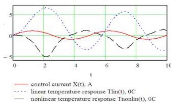
Fig. 3. Transients of the control current and temperature responses of the Peltier element in linear and nonlinear regime
