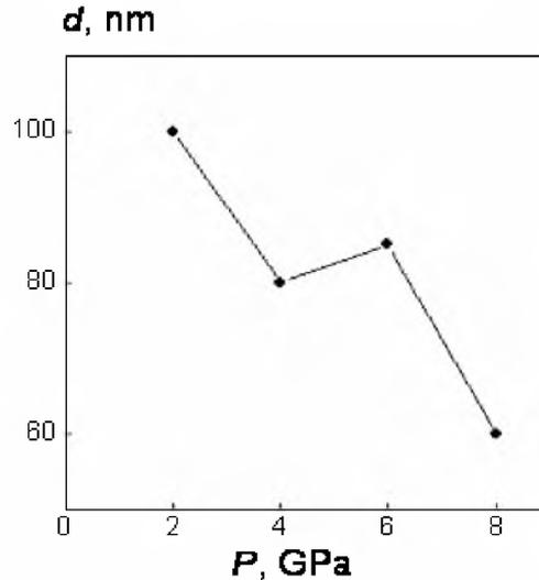
Fig. 4. The  $d(P)$  dependence for the Bi<sub>2</sub>Te<sub>3</sub>-based materials consolidated by the HIP method
