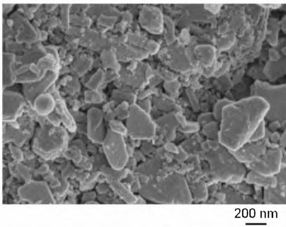
Fig 1. Morphology of the  $\text{Bi}_2\text{Te}_3$  nanopowder by SEM.
