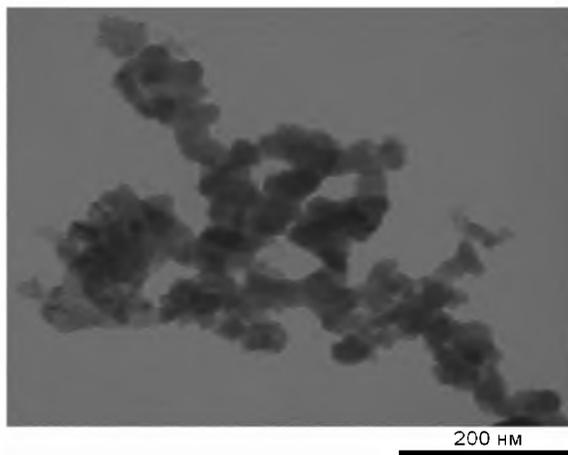
Fig. 2. Nanocrystals of the  $\text{Bi}_2\text{Te}_3$  powder by TEM.
