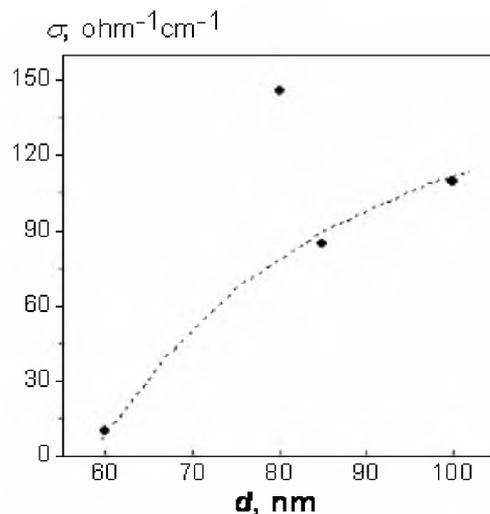
Fig. 5. The  $\sigma(d)$  dependence for the Bi<sub>2</sub>Te<sub>3</sub>-based materials consolidated by the HIP method
