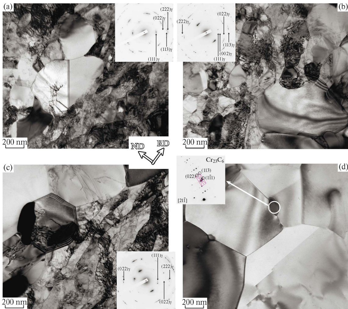
Fig. 3. Fine structure of the 304L steel after rolling at 200°C to \epsilon = 3 and subsequent annealing at 700°C for (a) 30, (b) 60, (c) 120, and (d) 480 min.
