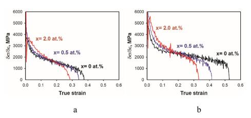
**Fig. 10.** Strain hardening curves of the CoCrFeMnNi alloys with different carbon contents (x): x = 0, 0.5, 2.0 at.% after cold rolling and annealing at 800 °C obtained at room (a) and cryogenic (b) temperature.
