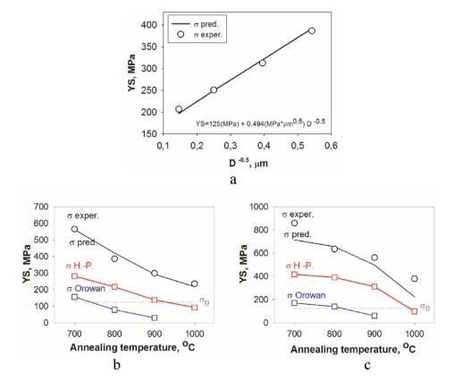
Fig. 13. Yield strength of the CoCrFeMnNi alloys with different carbon contents (x): x = 0 at % (a); 0.5 at % (b); 2.0 at % (c) depending on grain size (a) or annealing temperature (b,c).
