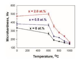
Fig. 1. Effect of annealing temperature on the microhardness of the CoCrFeMnNi alloys with different carbon contents (x): x = 0, 0.5, 2.0 at.%.
