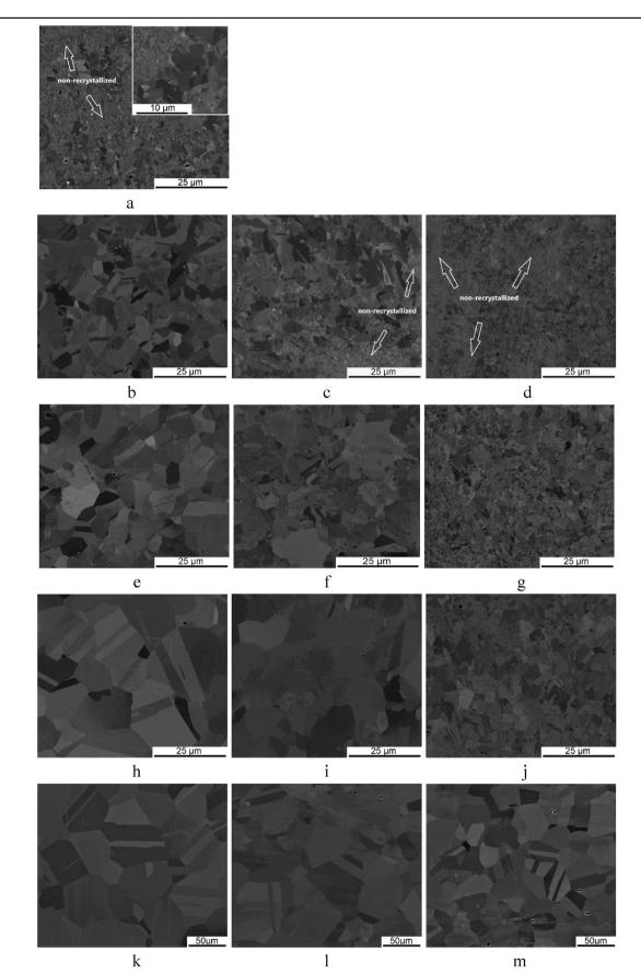
**Fig. 3.** SEM-BSE images of the microstructure of the CoCrFeNiAn alloys with different carbon contents (x): x = 0 at.% (a,b,e,h,k); 0.5 at.% (c,f,i,l); 2.0 at.% (d,g,j,m) after annealing at 600 °C (a); 700 °C (b-d); 800 °C (e-g); 900 °C (h-j); 1000 °C (k-m).
