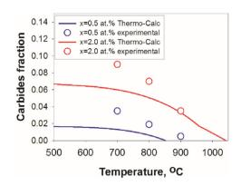
**Fig. 11.** Dependence of the equilibrium carbides fraction predicted by Thermo-Calc software in comparison with the experimental data in the CoCrFeMnNi alloys with different carbon contents (x): x = 0.5, 2.0 at%.
