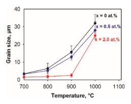
**Fig. 4.** Dependence of the recrystallised grain size on annealing temperature in the CoCrFeMnNi alloys with different carbon contents (x): x = 0, 0.5, 2.0 at%.
