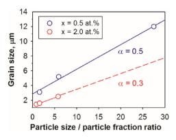
**Fig. 12.** Dependence of the fcc grain size on the particles size/fraction ratio in the CoCrFeMnNi alloys with different carbon contents (x): x = 0.5, 2.0 at.%. The dashed lines are only guides to eyes.
