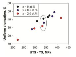
**Fig. 14.** The relationship between the ultimate tensile strength and yield strength difference and uniform elongation values in the CoCrFeMnNi alloys with different carbon contents (x): x = 0, 0.5, 2.0 at%.
