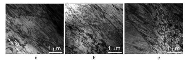
Fig. 2. Microstructure of the CoCrFeMnNi alloys with different carbon contents (x): x = 0 at % (a); 0.5 at % (b); 2.0 at % (c) after cold rolling to 80% thickness reduction; TEM bright-field images.
