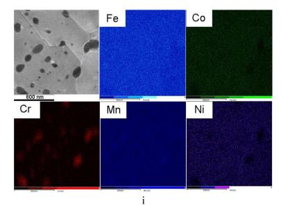
**Fig. 7.** TEM microstructure of the CoCrFeMnNi alloy with x = 2.0 at.% of carbon after annealing at 600 °C (a,b,c); 700 °C (d,e,f); 800 °C (g,i); 900 °C (h); bright-field images (a-h) and STEM image with corresponding EDX maps (i).
