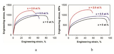
Fig. 9. Tensile stress-strain curves of the CoCrFeMnNi alloys with different carbon contents (x): x = 0, 0.5, 2.0 at.% after cold rolling and annealing at 800 °C (a) and 900 °C (b) obtained at cryogenic temperature.
