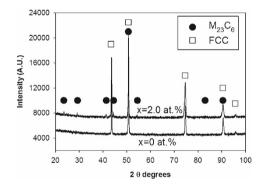
Fig. 5. XRD patterns of the CoCrFeMnNi alloys with different carbon contents (x): x = 0, 2.0 at  $\!\!\!\!\!\!\!\!\!\!\!\!\!\!\!\!\!\!\!\!\!\!\!\!\!\!\!\!\!\!\!\!\!$  after cold rolling and annealing at 800 °C.
