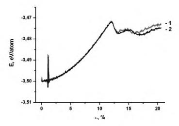
Fig. 4. Potential energy per one atom versus strain degree at 300 K for a compression rate of 50 m/s; scheme A (1) and Bain scheme (2).
