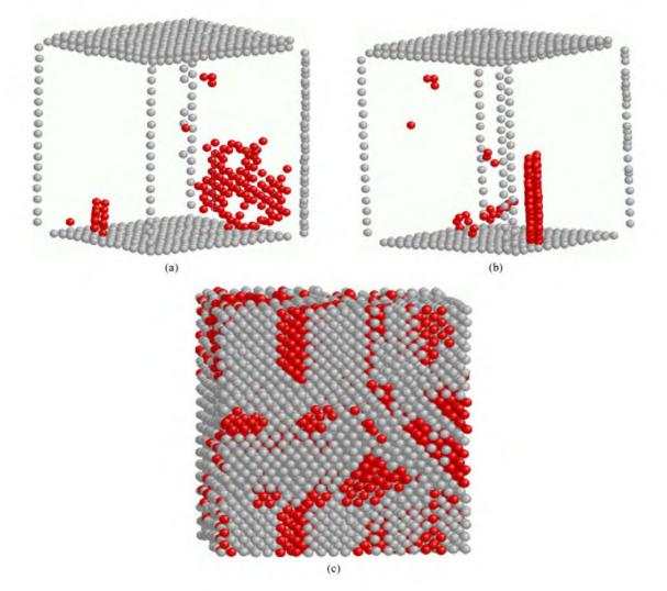
Fig. 2. Atomic structure at different view angles for the zone with local structural changes in compression by 11.3% along the Z-axis (a), (b). General view of the simulated crystallite in compression by 18% along the Z-axis (c); red spheres denote atoms belonging to the zone with local structural changes. (For interpretation of the references to colour in this figure legend, the reader is referred to the web version of this article.)
