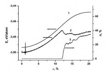
Fig. 1. Dependence of potential energy per one atom for 0 (1) and 300 K at a compression rate of 50 m/s (2); n—fraction of atoms with the topology of structural bonds, which corresponds to the HCP lattice (3).
