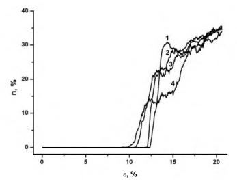
Fig. 3. Fraction of atoms (*n*) with the topology of structural bonds, which corresponds to the HCP lattice, versus strain degree for different temperatures of the crystal: 100(1); 300(2); 500(3); 700 K (4). The compression rate along the Z-axis is 50 m/s.
