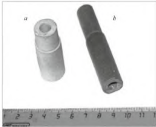
Fig. 3. Experimental items made of ceramic materials based on: a ) quartz sand powder; b ) sandy opoka powder.
