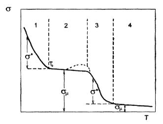
Fig. 1. The generalized plan of temperature dependence of a flow stress in polycrystallic metals (explain in the text).
