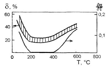
Fig. 3. The temperature dependence of the relative elongation of AISI304 and AISI316 steels irradiated up to fluence  $3 \cdot 10^{24}$  neutron/m<sup>2</sup> (dotted area) and  $\partial \sigma / \partial T$  that is the slope angle of flow stress temperature dependence in an unirradiated state.
