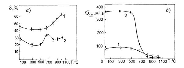
Fig. 2. Temperature dependence of a relative elongation (a) and yield strength (6) of nickel. 1 - unirradiated, 2 - irradiated up to a dose  $10^{25}$  el /m<sup>2</sup>.
