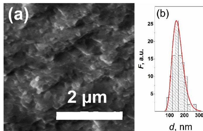
**Figure 3.** Typical microstructure of the fractured surface for the bulk  $(\text{BiSbSe}_{1.5}\text{Te}_{1.5})_{0.7}\text{Cu}_{0.3}$  sample (a) and the histogram of grain size distribution (b).
