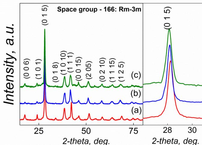
**Figure 1.** The XRD patterns of the  $\text{BiSbSe}_{1.5}\text{Te}_{1.5}$  (a),  $(\text{BiSbSe}_{1.5}\text{Te}_{1.5})_{0.7}\text{Cu}_{0.3}$  (b),  $(\text{BiSbSe}_{1.5}\text{Te}_{1.5})_{0.4}\text{Cu}_{0.6}$  (c) powders.
