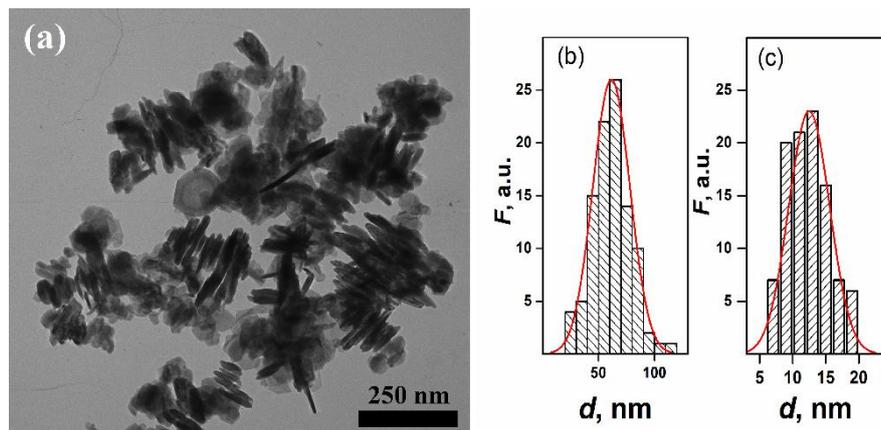
**Figure 2.** The TEM-image of the  $(\text{BiSbSe}_{1.5}\text{Te}_{1.5})_{0.7}\text{Cu}_{0.3}$  powder (a) and histograms of the nanoparticles diameter size (b) and thickness (c) distributions.
