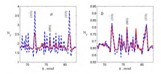
Figure 3: The same as on figure 2 c and d (solid lines) and the results of simulation neglecting the effect of scattering of the electrons on the thermal vibrations of atoms (dashed lines).
