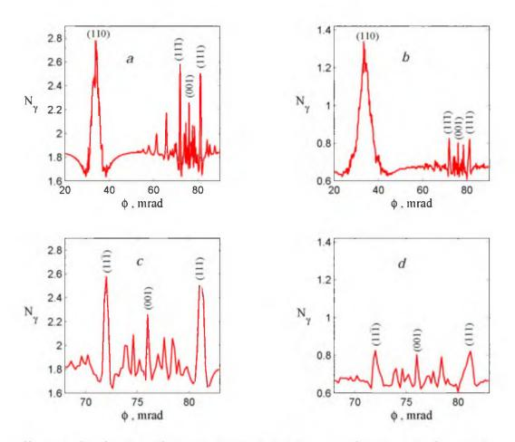
Figure 2: Results of simulation for the incoherent bremsstrahlung intensity (in ratio to Bethe-Heitler intensity in amorphous medium) from 855 MeV electrons in flat (left plot) and sinusoidally bent (right plot) silicon crystals under scanning of the goniometric angle like in the experiment [10]. We can see characteristic structures similar to that on figure 1b, generated by different crystallographic planes.
