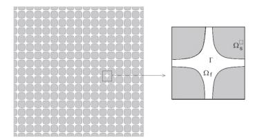
FIGURE 1. The pore structure
