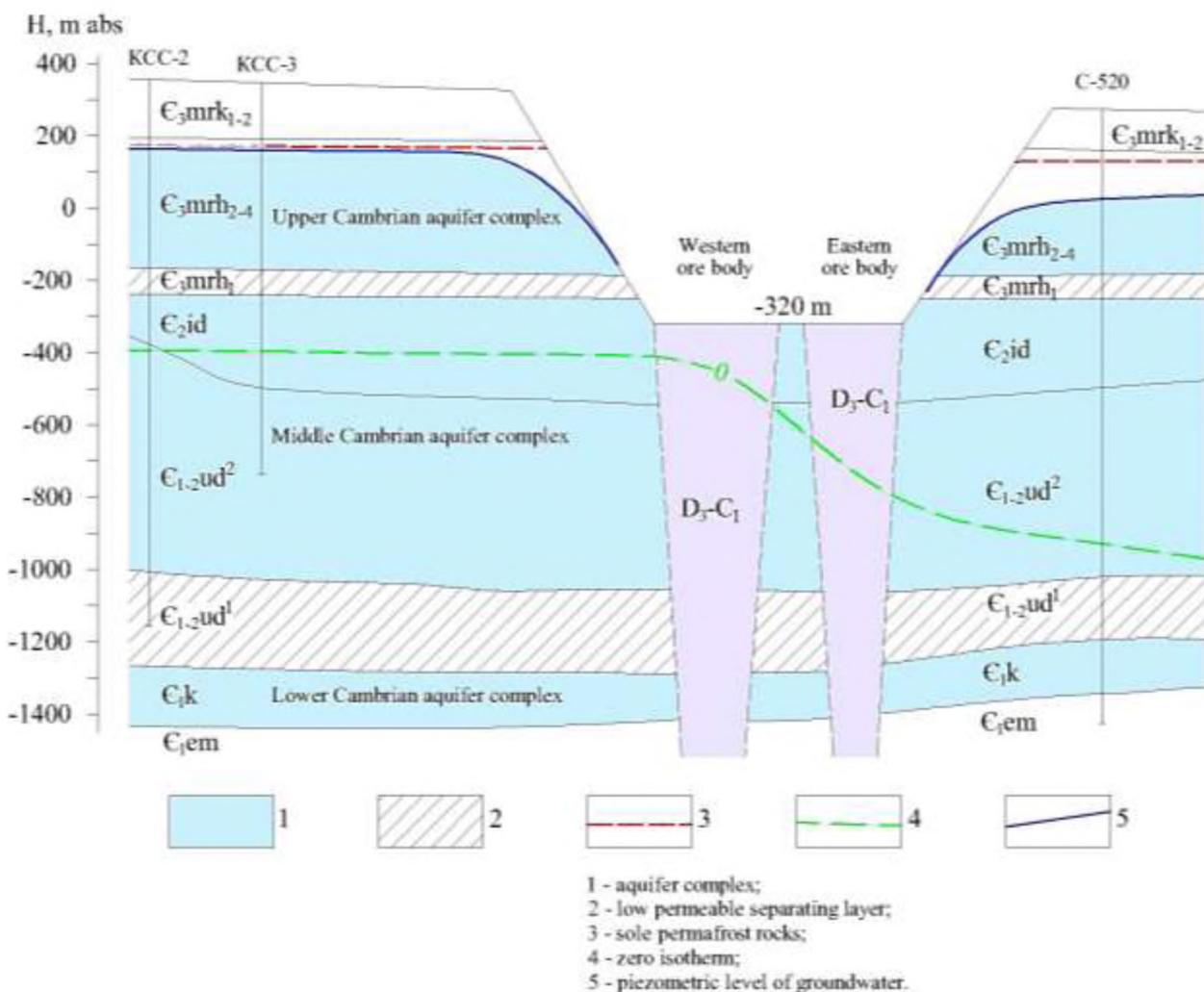
Fig.1: Cryohydrogeological schematic section through the Udachnaya pipe
