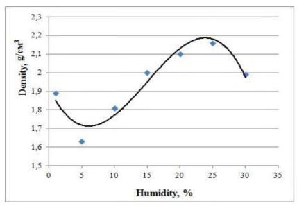
Fig.1: The dependence diagram of samples density of hydraulic filling mass against its humidity
