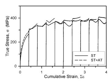
Fig. 1. True stress ( $\sigma$ ) vs cumulative strain ( $\Sigma\epsilon$ ) curves for the Cu – Cr – Zr alloy after solution treatment (ST) and solution followed by aging treatment (ST+AT). The multidirectional forging was carried out at 673K.
