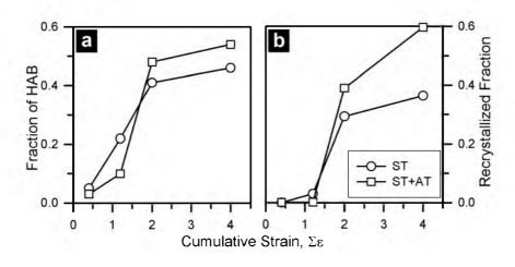
Fig. 4. The strain effects on (a) the fraction of high-angle boundaries (HAB) and (b) the recrystallized fraction in the ST and ST+AT alloys subjected to MDF at 673 K.
