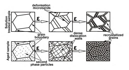
Fig. 6. Schematic illustration of the microstructure evolution in the Cu-Cr-Zr alloy during MDF at 673 K.
