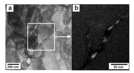
Figure 4. STEM micrograph (a) and Cr element mapping (b) of samples subjected to MDF at 600°C and then tensile tested at 500°C.
