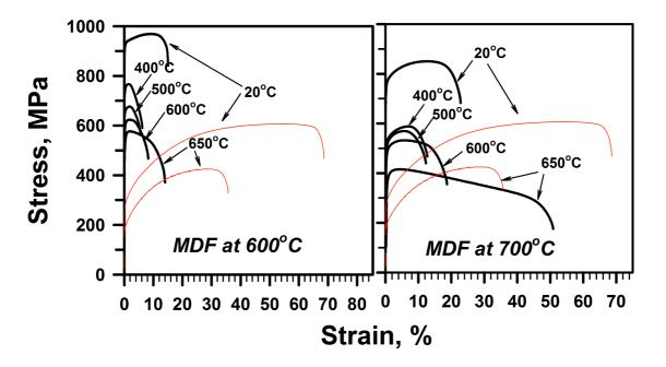
Figure 2. Tensile stress-strain curves of Super304H-type steel after MDF. The thin red lines correspond to the samples in heat treated condition.
