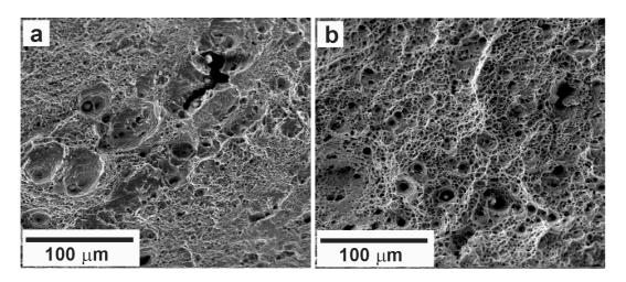
Figure 3. Fracture surfaces of samples subjected to MDF at  $600^{\circ}$ C and then tensile tested at  $500^{\circ}$ C (a) and  $650^{\circ}$ C (b).
