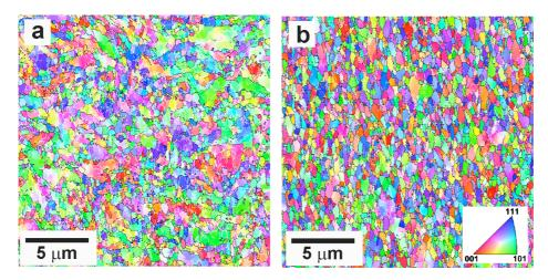
Figure 1. Typical OIMs of Super 304H-type steel after MDF (a) at 600°C, (b) at 700°C.
