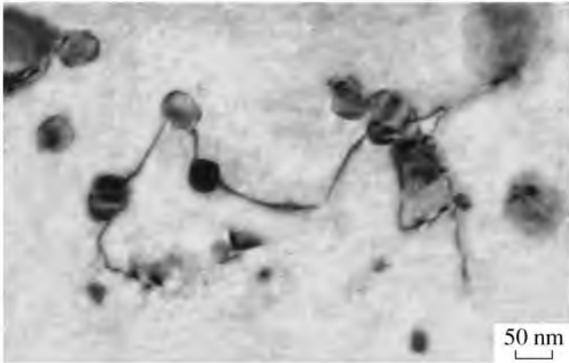
Fig. 4. Interaction of dislocations with dispersed particles in the Fe-0.6%O alloy after creep at 600°C at a strain rate \dot{\epsilon} = 1.3 \times 10^{-7} \text{ s}^{-1} .
