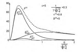
Fig. 9. Angular density of radiation in an asymmetrical case for higher electron energy than in Fig. 8.
