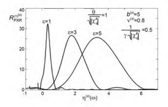
Fig. 3. Effect of reflection asymmetry on the PXR spectral width.
