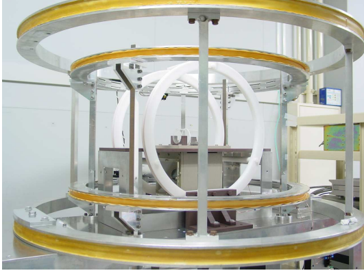
Figure 2: View of CNS polarized ^3\text{He} target [24] prepared for the experiment at Nuclotron-M.
